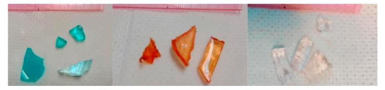
Figure 1 Hydrogels after the absorption of ions (from left to right) of copper, iron, and cobalt. A noticeable color change in the hydrogel is clearly visible due to the presence of the metal.
