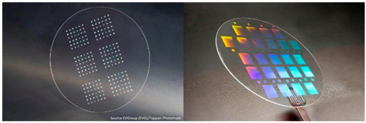
Fig.1 SmartNIL Imprint with meta-type lenses Fig 2. S&R master with augmented reality waveguides
